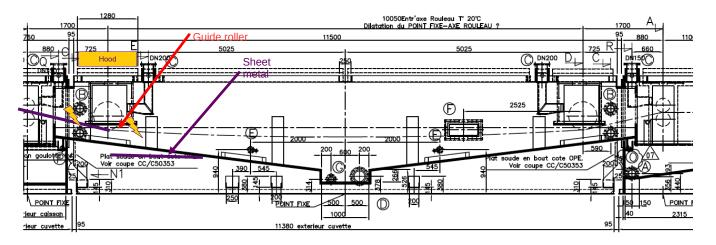
The tests performed by the plant operator revealed that the material surrounding the roller, i.e. EPDM (ethylene propylene diene monomer) rubber, only required a small amount of energy to ignite. Placing a match in immediate proximity would cause it to slowly burn and be consumed entirely.
