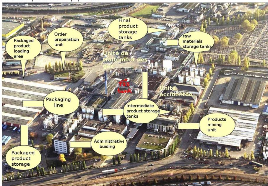
Fig. 2: Main plant installations (site operator)
